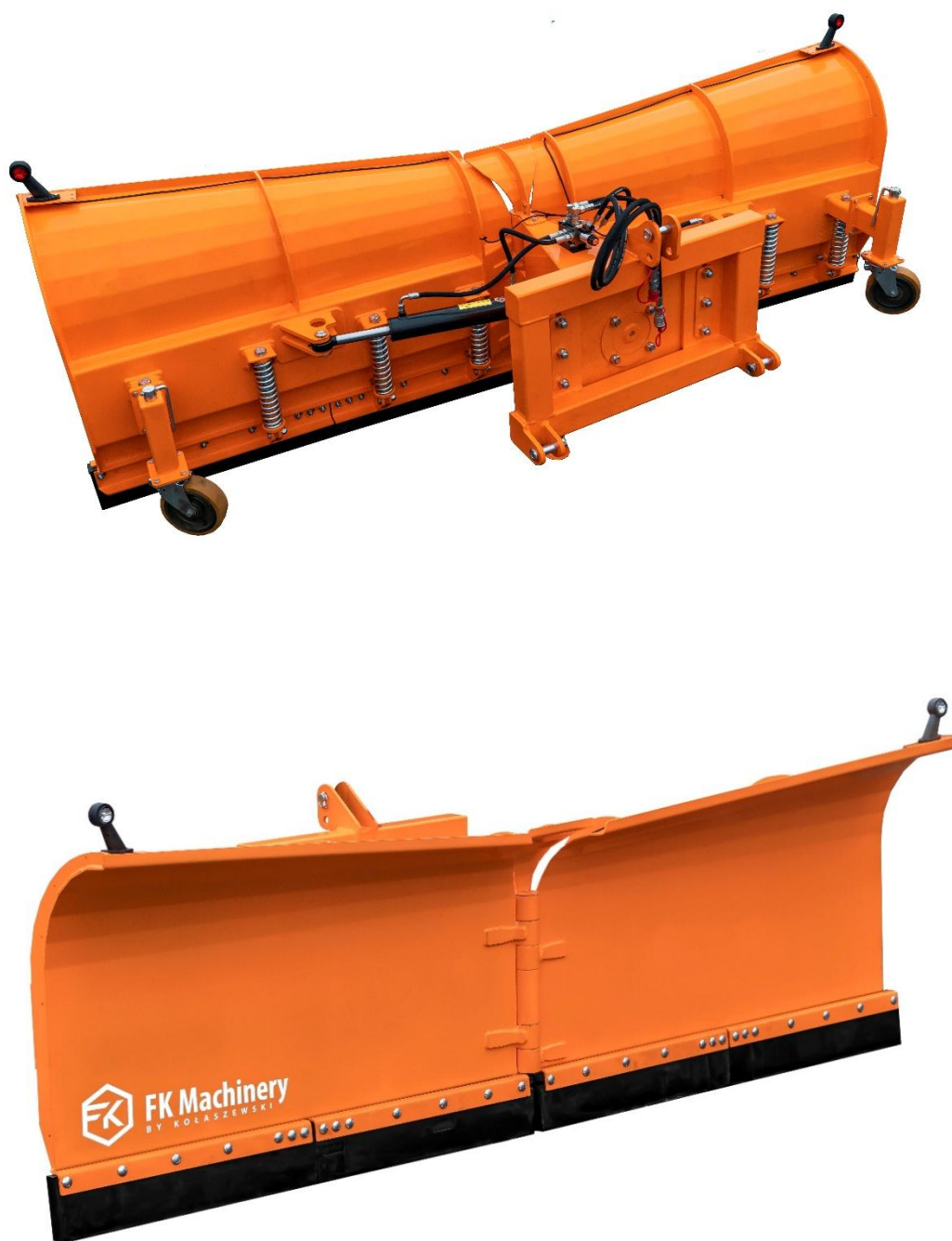
Fig. 1 General view of V-type snow ploughs.
